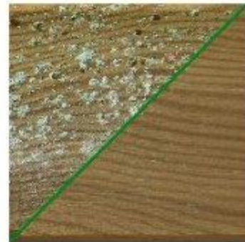
A light rub down with sandpaper, even the most severe case of speckling left by the treatment can be removed.
