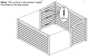
Turn the assembly upside down. Place the floor onto the bottom of the wall panels and secure in place using 6 x 60mm screws. Turn assembly up the right way once the floor is attached
