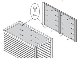
Turn the assembly up the right way and place the lid on top. Secure at the back using three hinges and 6 x 20mm screws per hinge. Open the lid and fix the lid stay using 1 x 40mm screw to the inside of the lid frame as show. On each side attach a chain to the inside frame of the lid and side panel using 2 x 12mm
