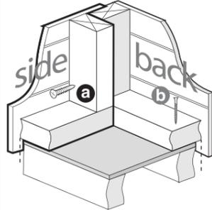
Position the panels so there is equal spacing in between the floor and the cladding on all 4 sides.
