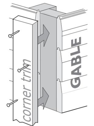
Please note corner / cover trims may need on site adjustment, cut with wood saw to appropriate size. Position corner trims level with bottom of building and fix with 3 x 30mm screws per corner. Position cover trims over joint where the two side sections meet and fix in same manner.
