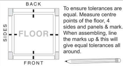
To ensure tolerances are equal. Measure centre points of the floor, 4 sides and panels & mark. When assembling, line the marks up & this will give equal tolerances all around.
