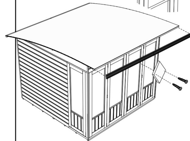
Using 2x40mm screws attach the finial to the centre of the fascia.
