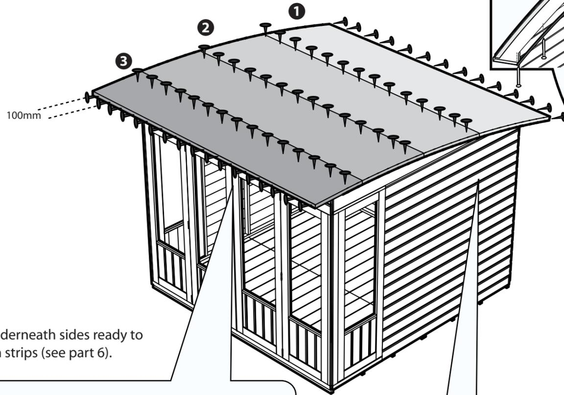
Fold felt underneath sides ready to secure with strips (see part 6).
