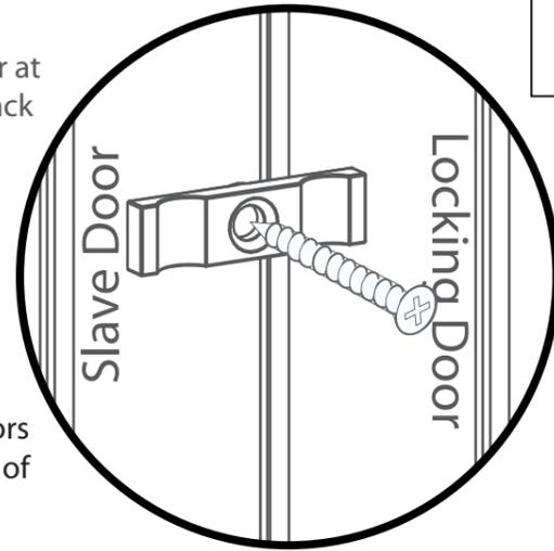
These turn buttons help to keep your doors straight during high levels and low levels of moisture content in the air.
