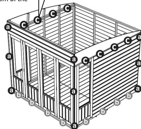
This building will distort if not erected on a firm and level base. Square the building to the floor, making sure the door and windows open.
