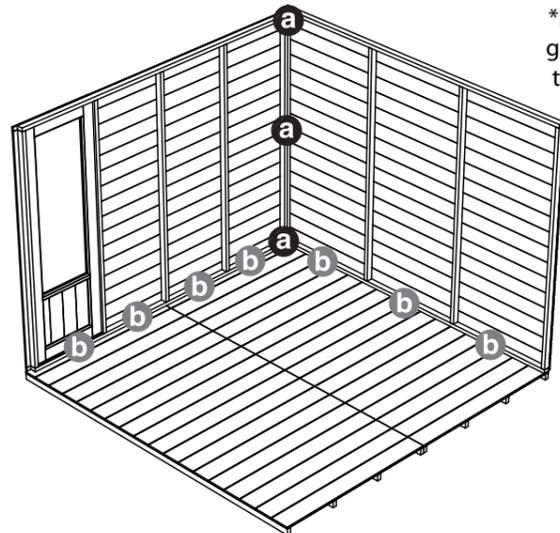
Position the rear gable onto the floor, the frame sits onto the floor with the T&G boards overlapping. Locate the side panel & rear gable frame to frame as in diagram.
