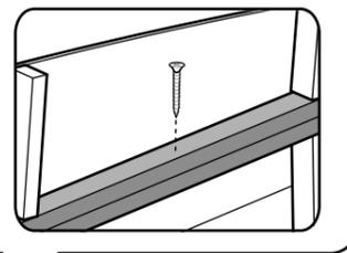
\*Important, Before fixing door gable, remove screws securing the doors from bottom of the panel
