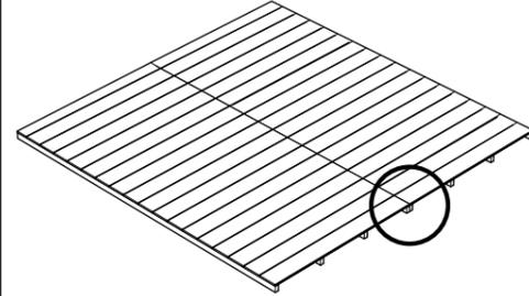
Position floor section a & b as in diagram so that floors are flush to each other, note that the floors do not connect by a T&G joint. Fix with 8x50mm screws alternate the fixing positions along the length of the floors
