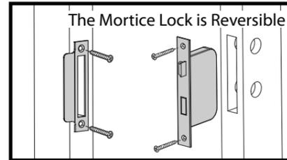
Fix Door handles and metal bar (spindle) using 8x 30mm screws. Ensure Mortice lock closes correctly. If not remove lock and turn catch around using small grub screw.
